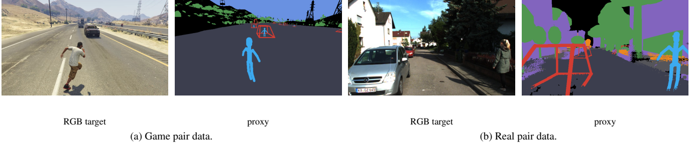
Fig. 3. Paired data construction. Each adjacent RGB–proxy pair is aligned at the same frame. (a) For game data, code reads structured runtime annotations to automatically produce pixel-wise, instance-level proxy annotations and preserve identity across frames. Note that, to ensure that the coding agent can easily reproduce the proxy at inference time, we exclude skeletal pose, detailed 3D models, and other representations that are difficult for coding agents to construct and maintain. Because extraction and compilation are code-based, a coding agent can easily add or revise the retained annotation channels through small, local program changes. (b) For real data, calibrated 3D reconstruction and object annotations compile the aligned proxy offline, preserving scene layout, entity locations, and occlusion without action labels or access to game-engine runtime state.
